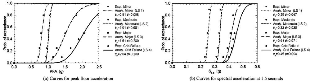
**Figure 11.** Fragility curves for configuration 1: undersized tiles. (a) Curves for peak floor acceleration; (b) Curves for spectral acceleration at 1.5 seconds.
