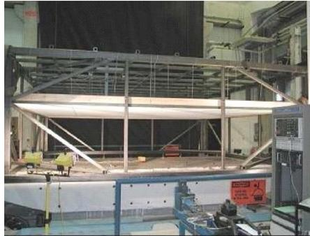
**Figure 1.** Test fixture mounted on the simulator at the University at Buffalo.
