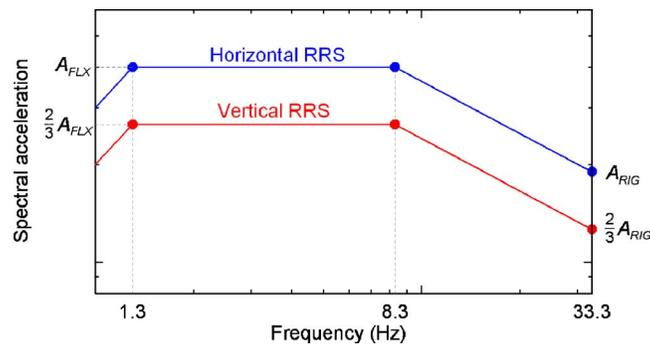
**Figure 5.** Required response spectra (RRS) for horizontal and vertical shaking (adapted from ICC, 2004).
