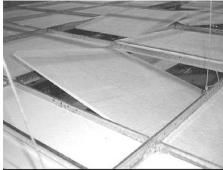
**Figure 7.** Tile rotating before falling, configuration 1.
