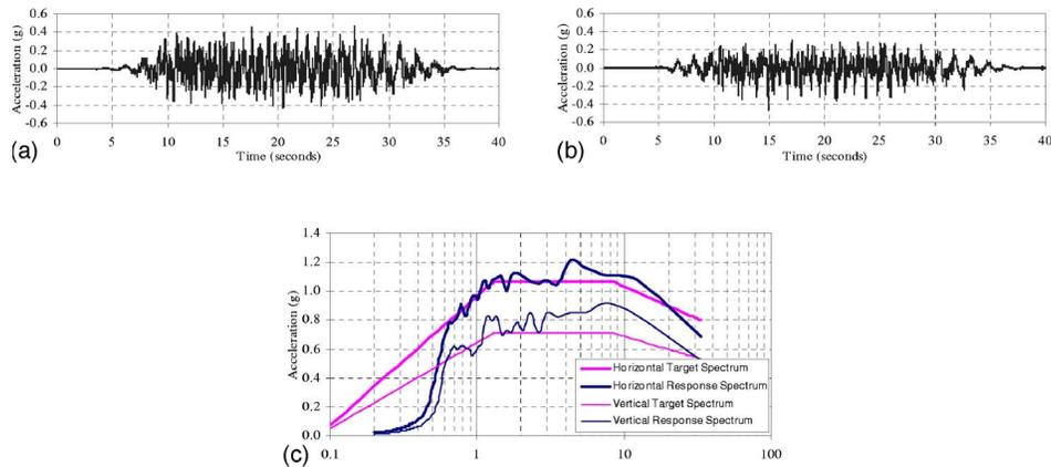
**Figure 6.** Earthquake histories and spectra for a level of shaking corresponding to  $S_5$  equal to 1.0 g. (a) horizontal acceleration; (b) vertical acceleration; (c) horizontal and vertical response spectra (target and calculated).
