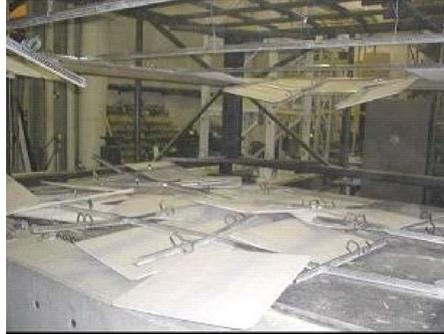
**Figure 9.** Failure of grid and tiles in configuration 5.
