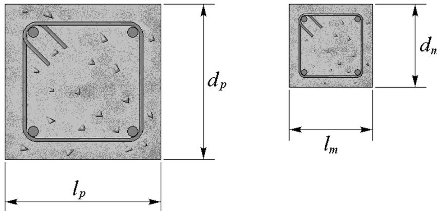
$$\frac{l_p}{d_p} = \frac{l_m}{d_m} \quad \text{so} \quad \frac{A_p}{A_m} = \left(\frac{d_p}{d_m}\right)^2 = \left(\frac{l_p}{l_m}\right)^2$$
